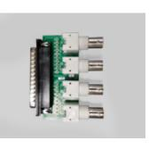
ADP-BNC P/N: 32952001 D-sub to BNC adapter board
